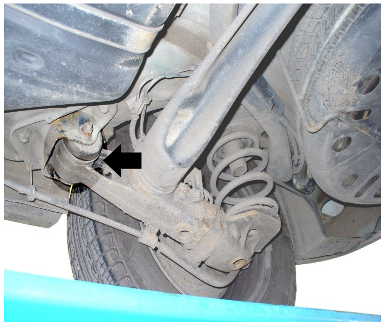
Figure 15. Bearing elements of longitudinally directed support rods
